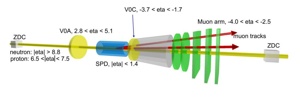
Muon Arm and trigger detectors
