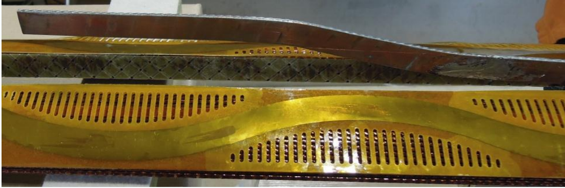
Stainless steel Quench Heaters for magnet MQXC(+2m long)
