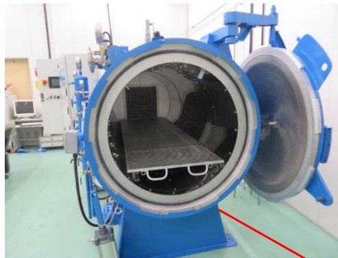
New autoclave 2.5m x 1m
