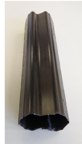
Production of Shell longeron prototypes for ATLAS phase 2 pixel upgrade (SLIM)
