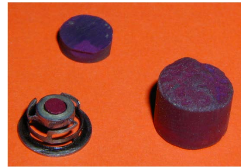
cathodes damaged by sputtering
