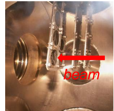
Carbon foil at CERN LINAC3
