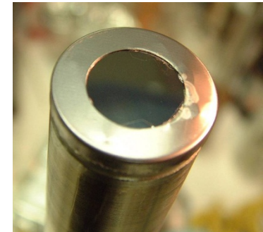
Stalk for supporting 1 Photocathode
