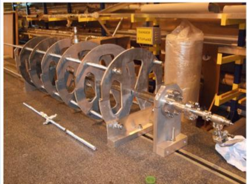
Figure 4: Test set-up of the vacuum chamber
