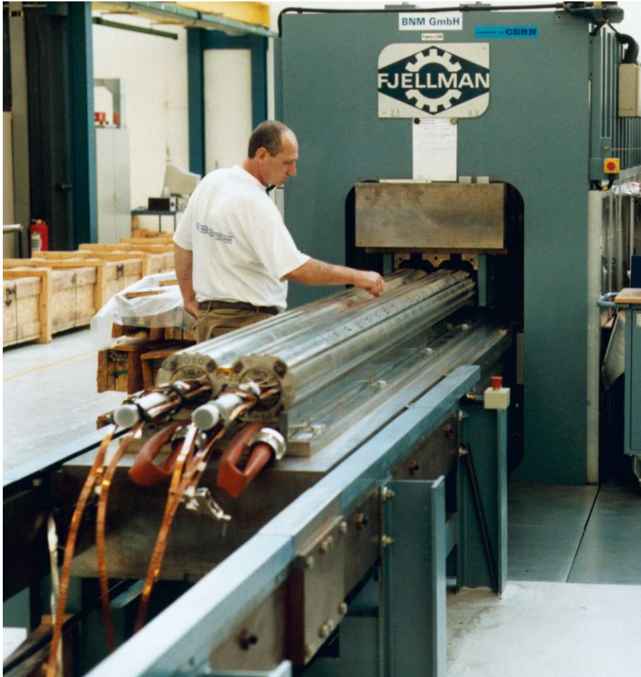
Collaring of a dipole magnet
