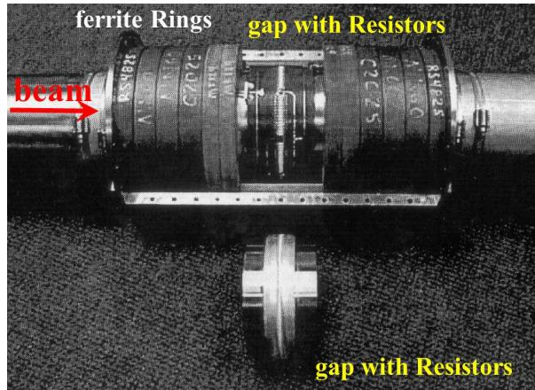
Figure 6.14: Photo of the wall current monitor used at FERMI-Lab for protons, from [119]. The ceramic gap is shown separately. The ferrite rings and the printed circuit with the resistors are visible.
