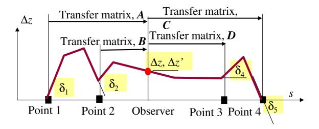
**Calculate the kicks**  $\delta_1$  and  $\delta_2$  to achieve the displacement  $\Delta z$ ,  $\Delta z'$  at the Observer position by using the steering equation (4.8).
