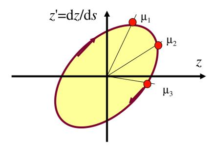
★ In the case of a ring or matched cell, the periodicity imposes equality on the input and output  $\alpha$  and  $\beta$ values. This means that the particle returns after each turn or transit to the same ellipse but at phases  $\mu_1 = B$ ,  $\mu_2 = B + 2\pi Q$ ,  $\mu_3 = B + 4\pi Q$ , ....,  $B + n2\pi Q$ and so on.
