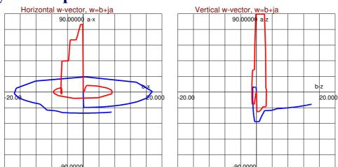
Correction of a half a DBA cell. Blue curves are open showing w-vectors entering straight section. Red curves are closed and go to zero.
