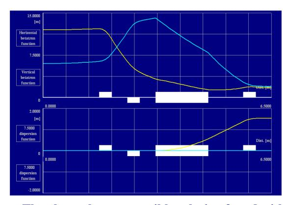
The above shows a possible solution found with WinAGILE. The input ratio  $\beta_z$  /  $\beta_x$  is around 0.5, which is characteristic of one family of solutions. Other families with  $\beta_z \cong \beta_x$  or much larger or smaller values are also possible.
