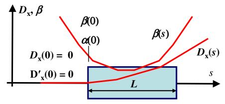
For a horizontal bending dipole, for which we neglected the weak focusing term  $1/\rho^2$ , but keep k,
