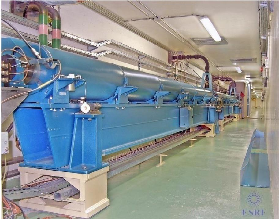
The Linac consists in one **TRIODE** (cathod – anod – grid) powered with 100 KV. Electrons produced have then an energy of 100 keV.
