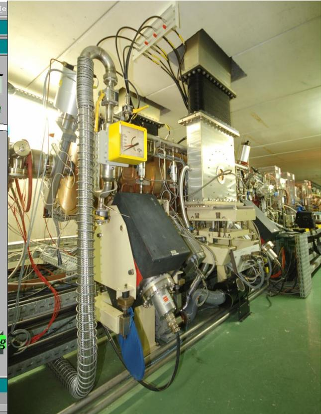
Goal: compensate the energy loss turn / turn by the electrons, following the synchrotron radiation emission, i.e., 4.8 MeV (with all insertion devices)
