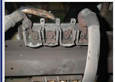
Magnet PS circuit breaker short circuit
