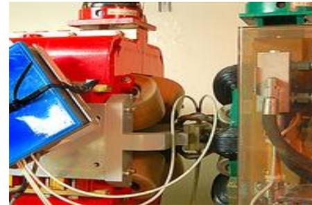
224 Beam Position Monitors to measure the positions of the electron beam center of mass in the horizontal et vertical planes
