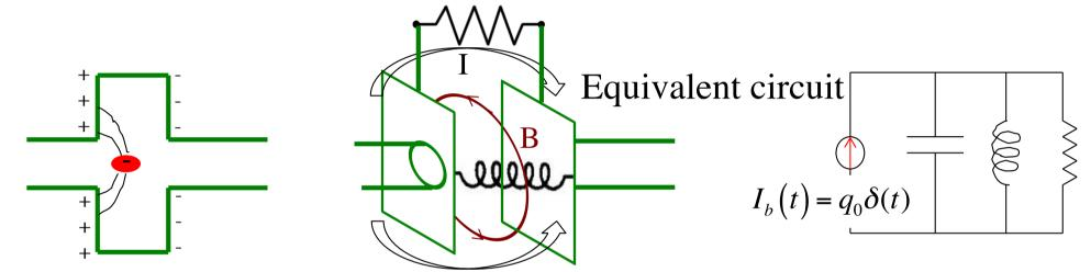
Each mode can be treated as an electric RLC circuit loaded by an impulsive current. Just after the charge passage, the capacitor is charged with a voltage  $V_o = q_o / C$  and the electric field is  $E_{so} = V_o / l_o$ .
