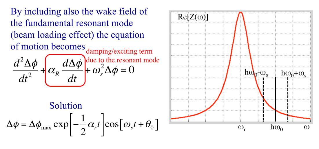
$$\alpha_r = \frac{eN_p \eta h \omega_0}{\omega_s (E_0 / q) T_0^2} \operatorname{Re}[\Delta Z]$$
