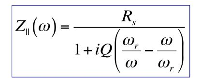
This impedance can be also used as a simplified impedance model of a whole machine for the short range wake fields assuming  $Q \sim 1$  (it is called **Broad Band Impedance Model**)
