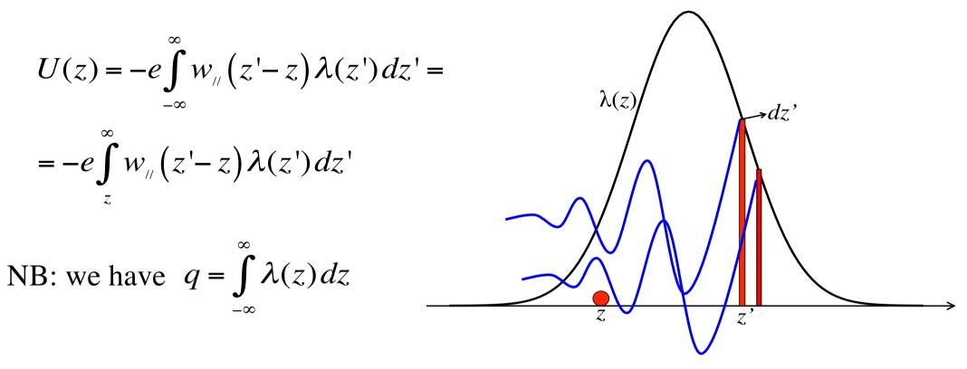
The energy lost allows to define the *longitudinal wake potential of a distribution*
