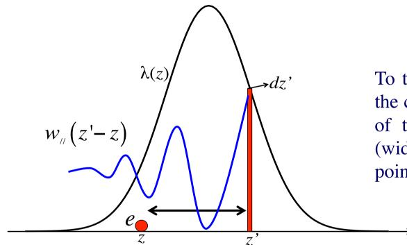
To this end let us evaluate the effect on the charge e in a posizion z due to a slice of the bunch in a position z' so thin (width dz') that it can be considered as a point charge:
