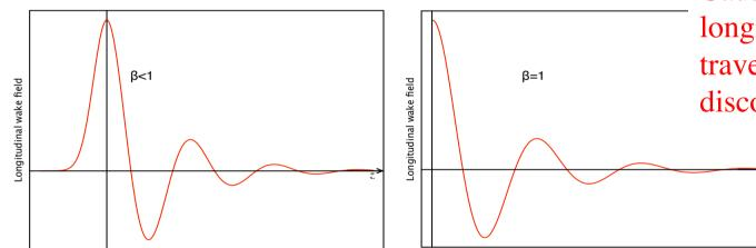
Causality requires that the longitudinal wake field of a charge travelling with the speed of light is discontinuous in the origin.
