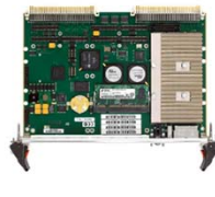
VME Card: Eurocard size VMEbus interface
