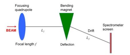
3.1 If the effective length of the dipole is  $l_B = 0.43$  m, what should be the magnetic field (in Tesla) inside the dipole to deflect the electrons by an angle of 35 degrees?
