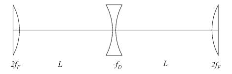
This exercise considers a general case where  $f_F$  is not necessarily equal to  $f_D$ . Using the thin lens approximation for the FODO cell with drifts of length L we get the following matrix:
