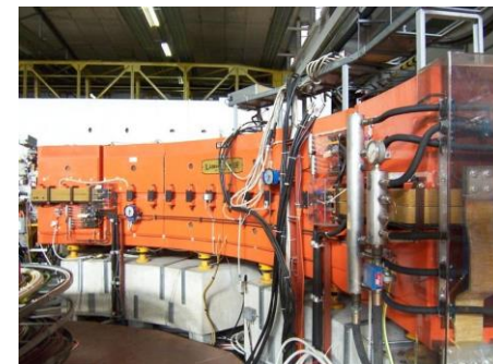
LEIR main dipole, 60 tons
