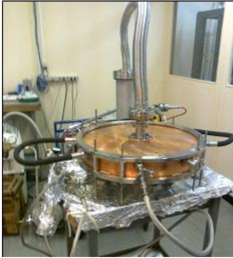
Leak and pressure test of PIMS disks
