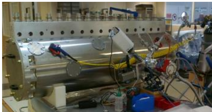
Leak and pressure test of PIMS disks
