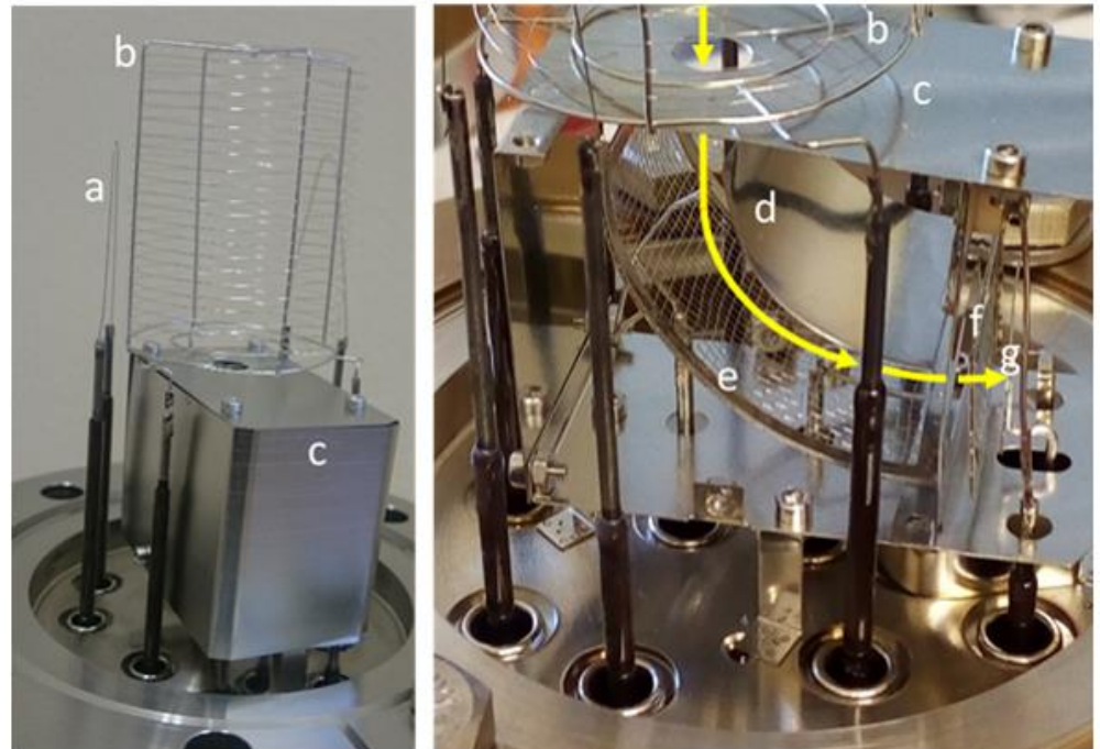
Figure 8: Main components of the Helmer gauge; on the right with opened cage. (a filament, b grid, c cage, d inner deflector, e outer deflector (on ground potential), f suppressor, g collector). The yellow line indicates the ion trajectory from the grid volume towards the collector.
