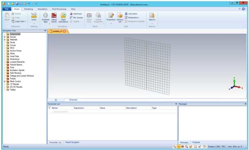
The working window is divided into 5 sub-windows (but it depends on the chosen preferences). The largest one shows the figure of the device you are designing.
