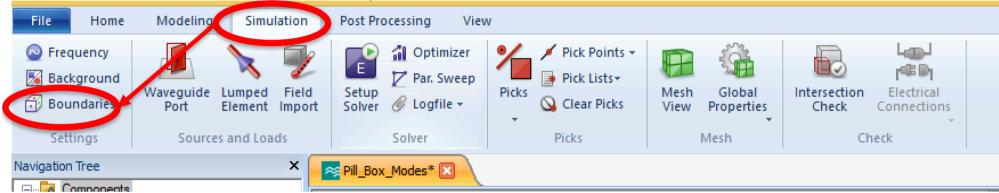
Let's now select the simmetry planes of our geometry from the "Symmetry Planes" window (YZ Ht=0 and XZ Ht=0) and the boundaries as shown below.
