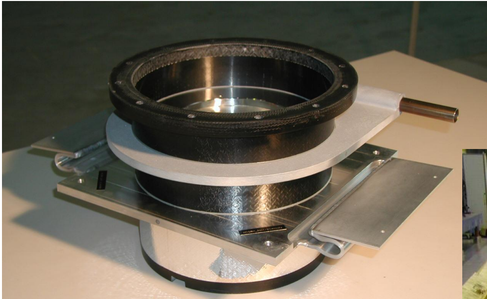
Low heat inleak GFRE support post
