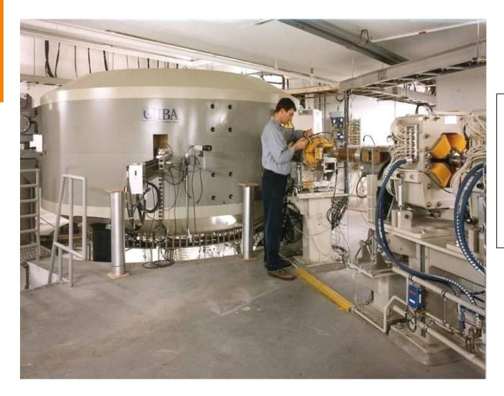
Protons only Fixed energy 200 tons  $\emptyset = 4.7 \text{ m}$
