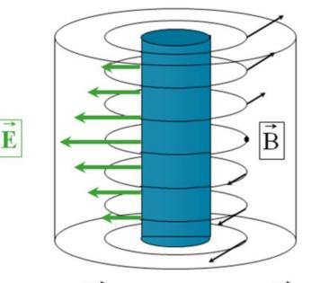
Electric (E) and magnetic (B) fields in Rhodotron coaxial cavity
