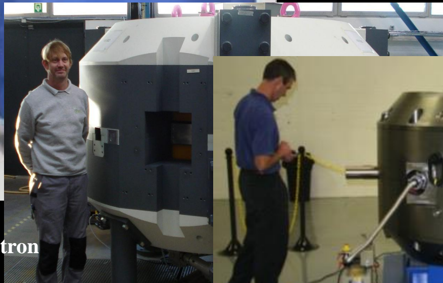
IBA – 50 Ton Synchrocyclotron
