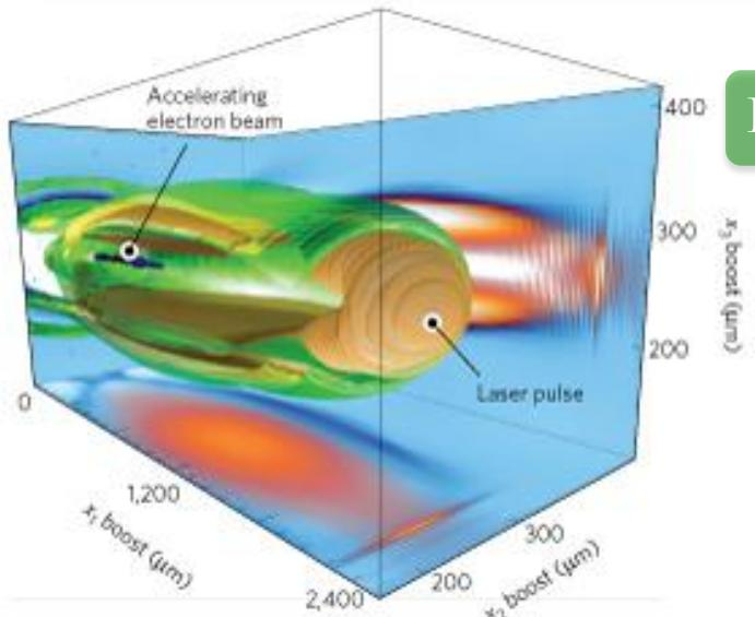
Laser-wakefield electrons to trigger the cascade in a solid
