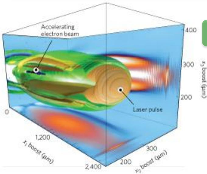
Laser-wakefield electrons to trigger the cascade in a solid
