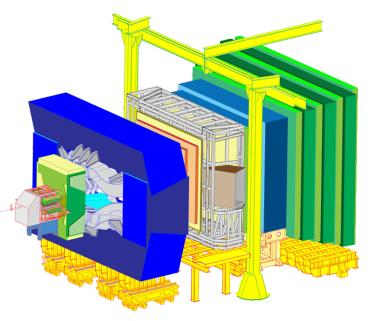
General purpose detector optimized to measure *b*-hadron pairs produced in the forward region from pp or HI collisions at the LHC
