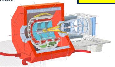
General purpose detector optimized for the high-multiplicity environment of HI collisions at the LHC. Complementary to other LHC experiments due to low- $p_T$ threshold and excellent PID capabilities
