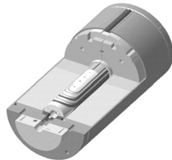
Fig. 4. Cross-sectional view of 56-mm-aperture, 210-T/m Nb 3 Sn quadrupole magnet model under development at CEA/Saclay.
