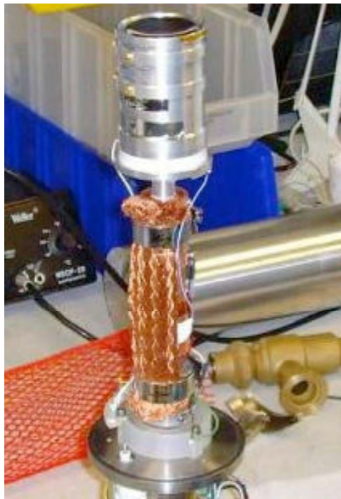
n-type, natural HPGe detector before LAr immersion tests
