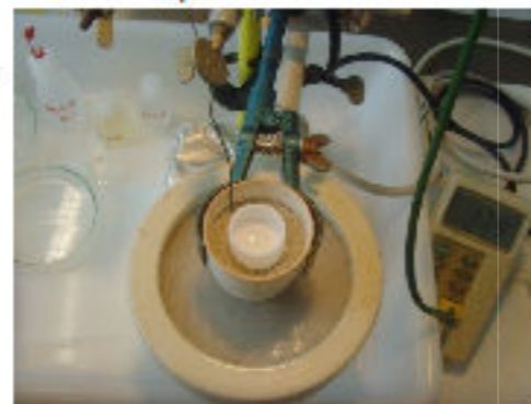
Adding nitric acid to the ^{228}\text{ThCl}_4 solution
