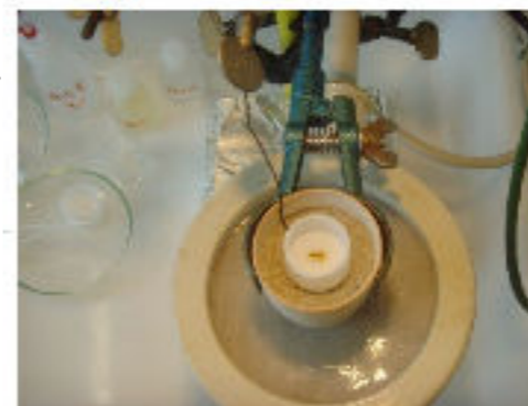
Refilling ^{228}\text{Th}(\text{NO}_3)_4 into the goldcrucible
