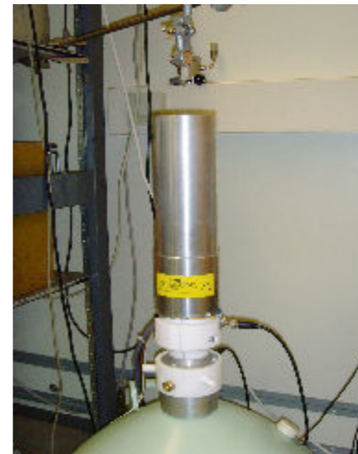
HPGe detector in UZH lab (here operated in vacuum)
