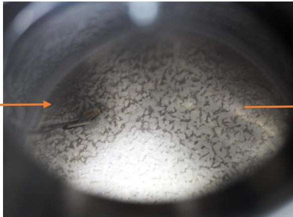
Outside of core, condensed Flammable gasses and grown sD 2 crystals this year
