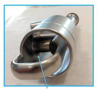
Maximum excessive weld metal penetration measured 0.3mm
