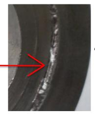
1 local defect found in the overlap Undercut measured: 1.7mm
