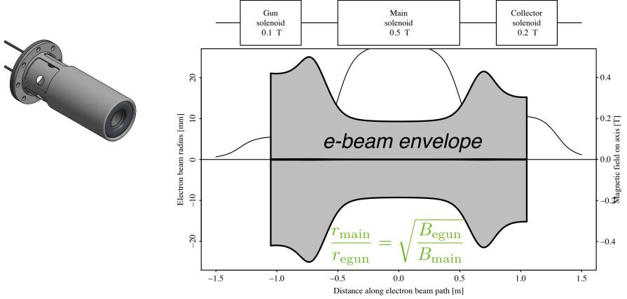
For 20 A and a 50% active area, a radius of 32 mm is required with barium-oxide dispenser cathodes
