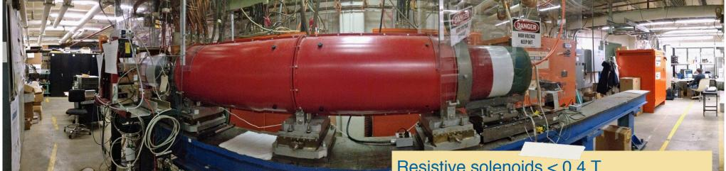
Resistive solenoids < 0.4 T Total length 2.8 m (straight configuration) 10 keV, 5 A electron beam 200 kW electrical power
