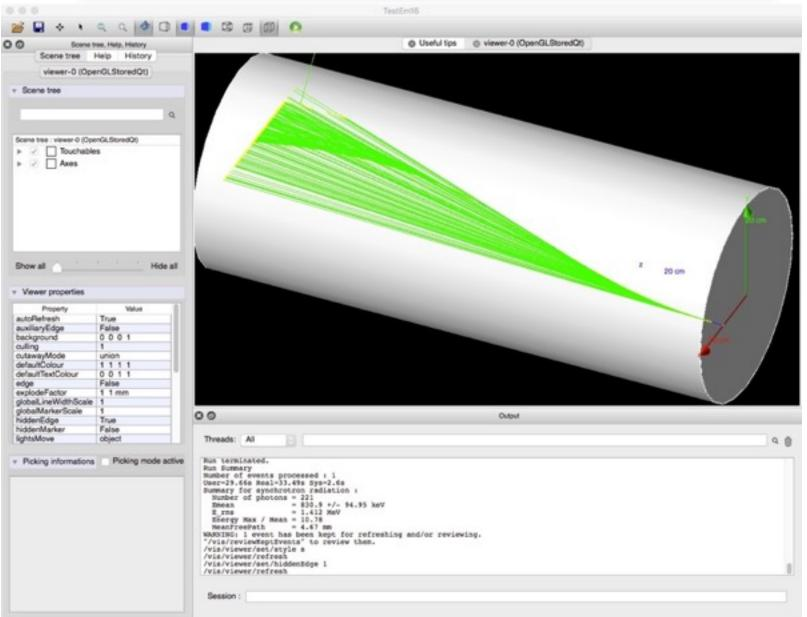
10 GeV e+, SingleQuad 500 T/m 1m long, 20 cm quad radius, 10 cm offset in x, SynRad on
