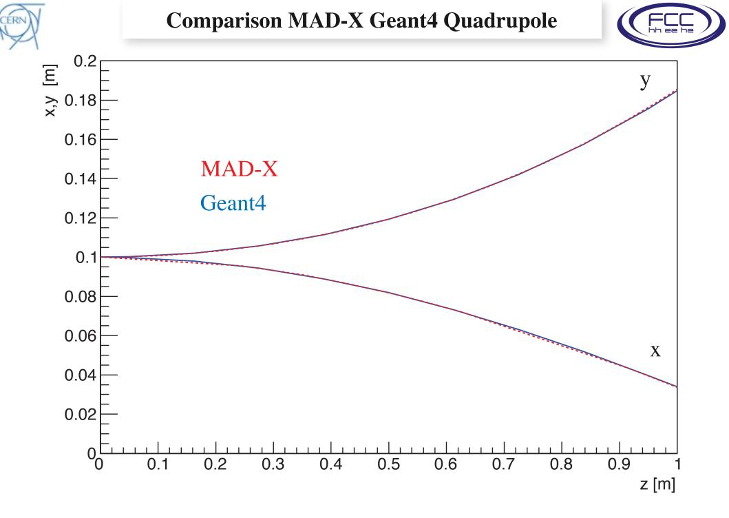
MAD-X : using MAKETHIN, 10 thick quadrupole slices to visualize trajectory in quadrupole
