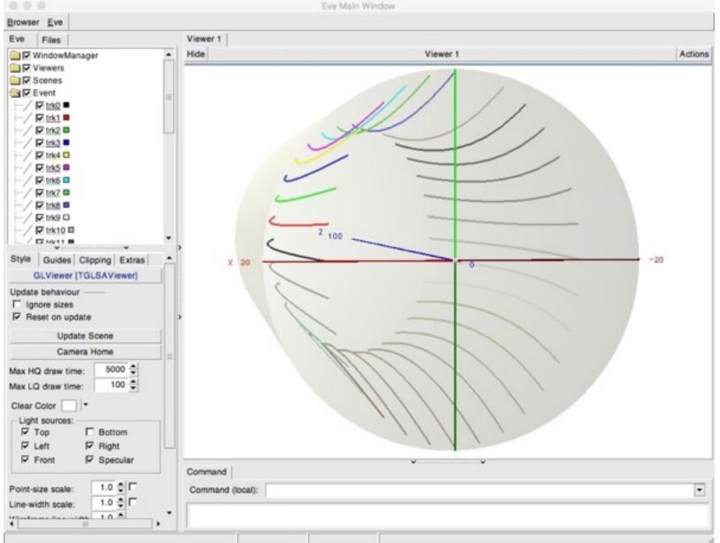
SingleQuad.madx + tracking + plotting in MDISim Focusing in x (curved to inside), defocusing in y. 500 T/m. 1m long, 20 cm quad radius, 16.5 cm offset.
