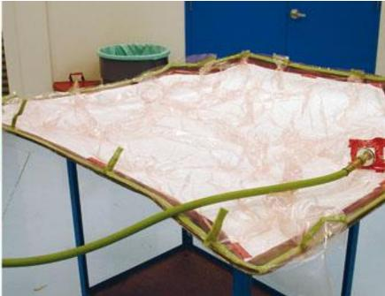
In a pleat: Allows placement on any mold, anywhere. However, the pleat must have adequate breather to ensure conduction to the bulk of the tool surface, and it should be strain relieved so as to aviod bridging of the pleat where it contacts the tool.
