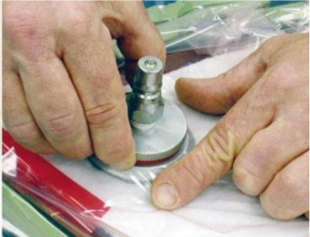
Close vacuum Fitting: There are ½ twist and threaded varieties of vacuum fitting. In both cases, make sure elastomer seal is outside the bag and against bag material. Stretch bag to ensure that there are no wrinkles against the foot of the vacuum fitting.
