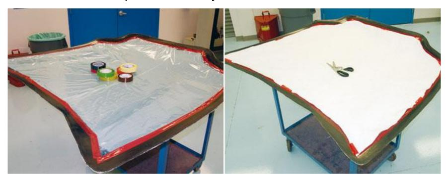
Release Film (Plastic Sheet): Can be loosely applied over peel ply, but must not bridge. Can be perforated or not. Prevents breather from becoming saturated with resin, starving laminate, and cutting off vacuum. Perforations allow for greater resin flow/loss. Need to experiment for rich or high-volatile systems.
