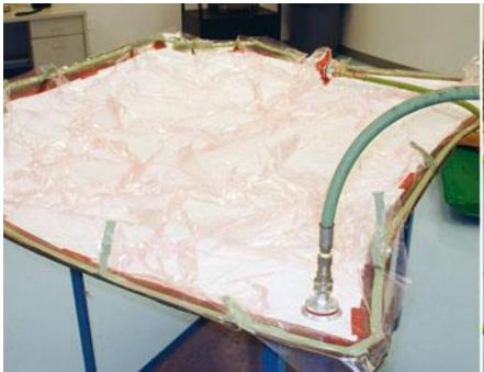
Against the mold surface is most secure: However, sometimes there is no space for the fitting, or applying to the mold (for example a curved mold) would cause bridging and potential bag failure.
