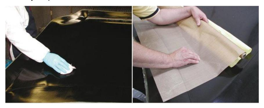
Release Agent (Wax): Good for any shape, but requires reapplication for every cure cycle. Must be applied properly, depends on tool material.
