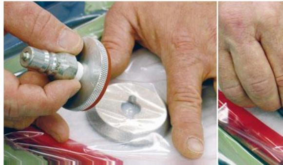
Foot of vacuum fitting must be inserted into bag:
