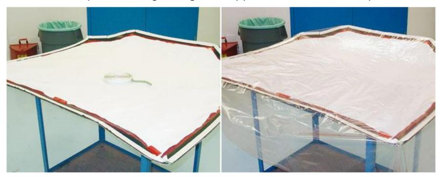
**Bag Sealant (« Tacky ») Tape:** Applied continuously to tool all the way around the part. Must be rolled onto tool for good seal. Can be doubled, but care should be taken to avoid penetrating leaks.
