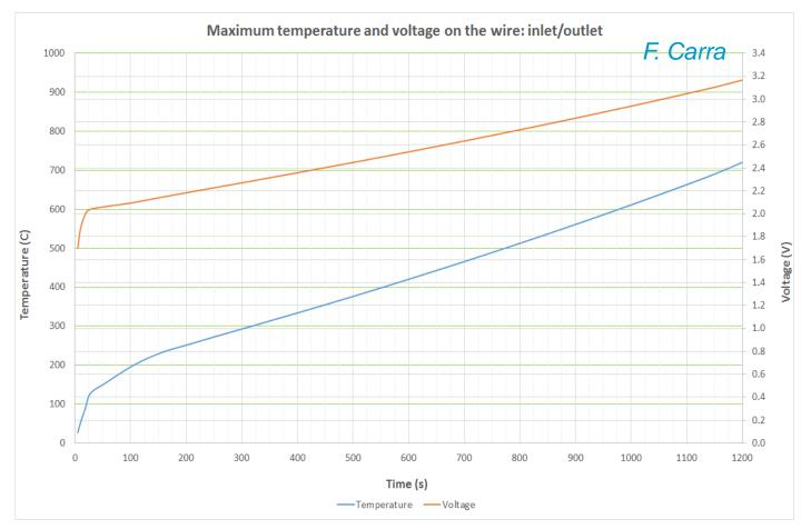
Time evolution of the wire temperature (blue line) at locations where it reaches maximum temperature; and of the corresponding voltage (red line) between the wire extremities, assuming a current of 378 A, no water-cooling in the jaw, no thermal losses due to radiation, only heat conduction
