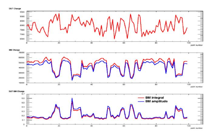
There is anti-correlation between the charge collected by the BM and the one collected by the DUT diode The signal on the BM was smaller when the bending radius of the optical fiber was shorter
