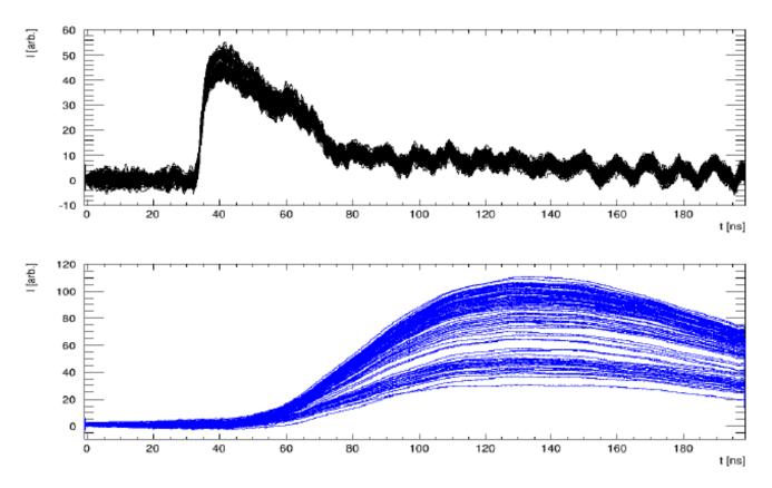
Both signals in the BM and in the DUT were quite small but the DUT was hit in the center 20ns to100ns as time interval for charge integration in the DUT
