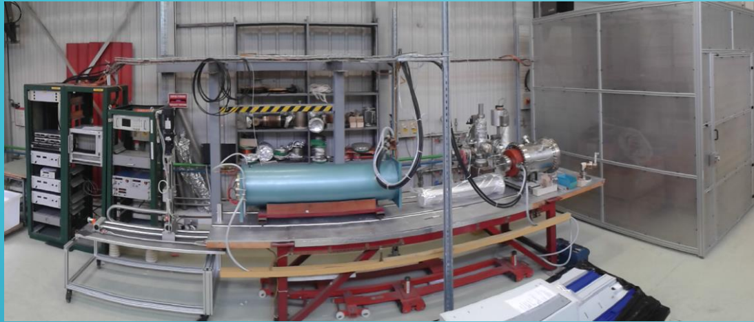
New gun tested on linear test stand (solenoid field of 100 G)
