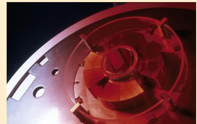
**LHC main quadrupole magnet**       $g \approx 25 \dots 220 \text{ T/m}$
