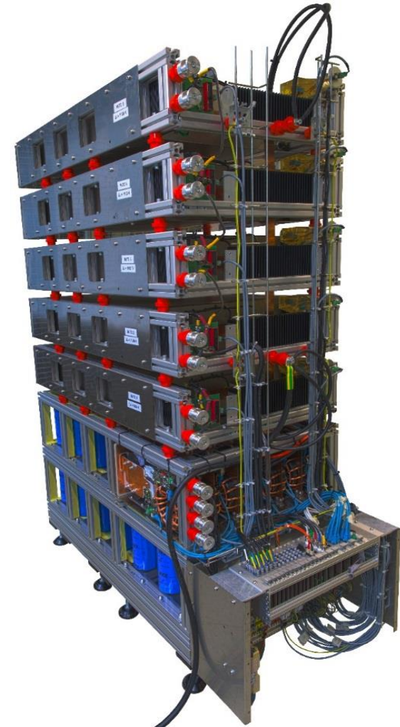
Photo of the first prototype of the modular current source. The prototype was designed and built at the HPE laboratory, ETH Zurich.
