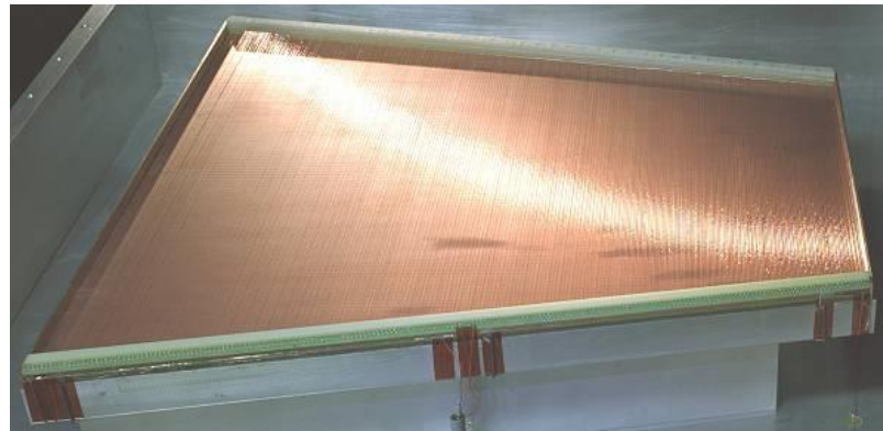
Wire chamber: 40 \mu m
