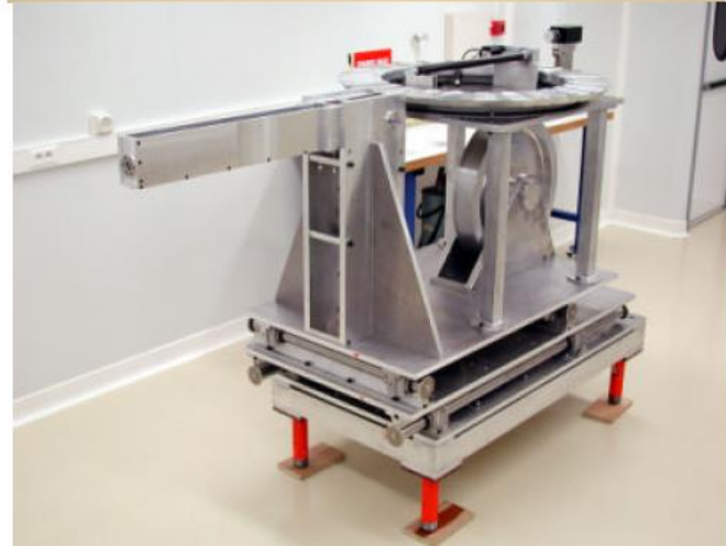
"Carousel" brick dispensing and storage system
