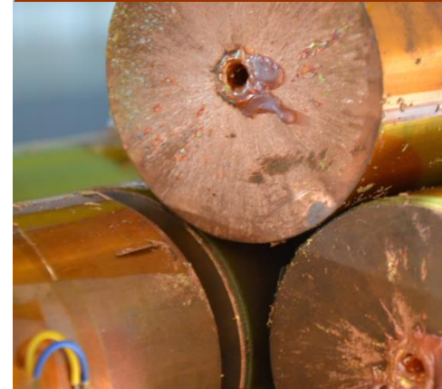
Damage of a beam with an energy of 2 MJ
