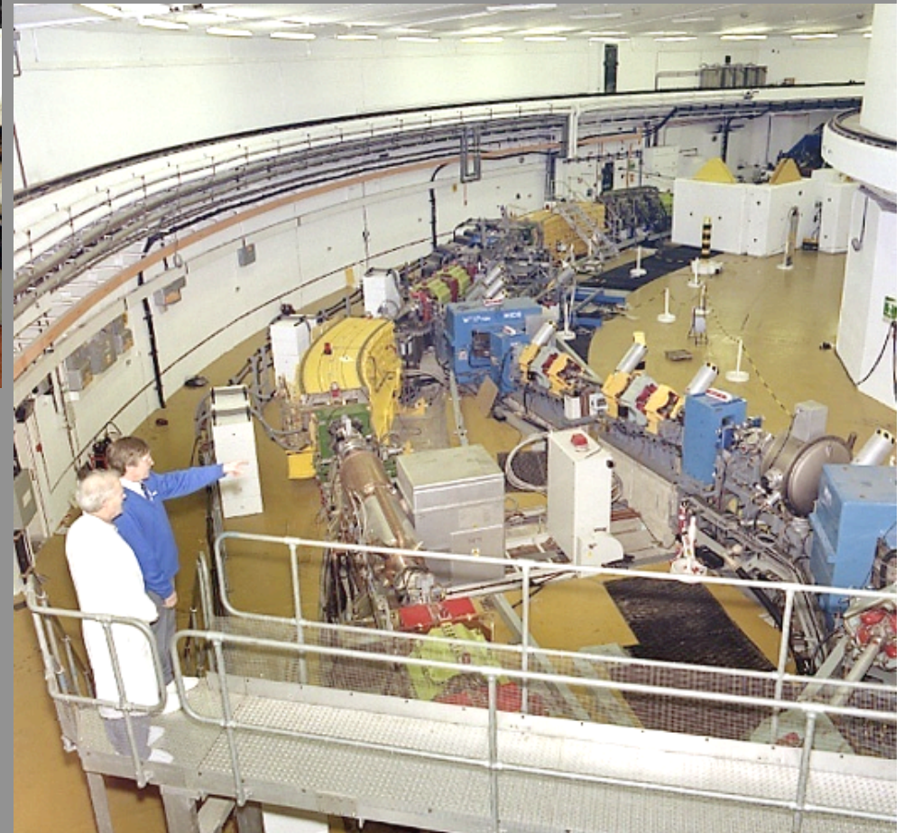
ISIS 800 MeV proton synchrotron 1.3–3.1 and 2.6–6.2 MHz
