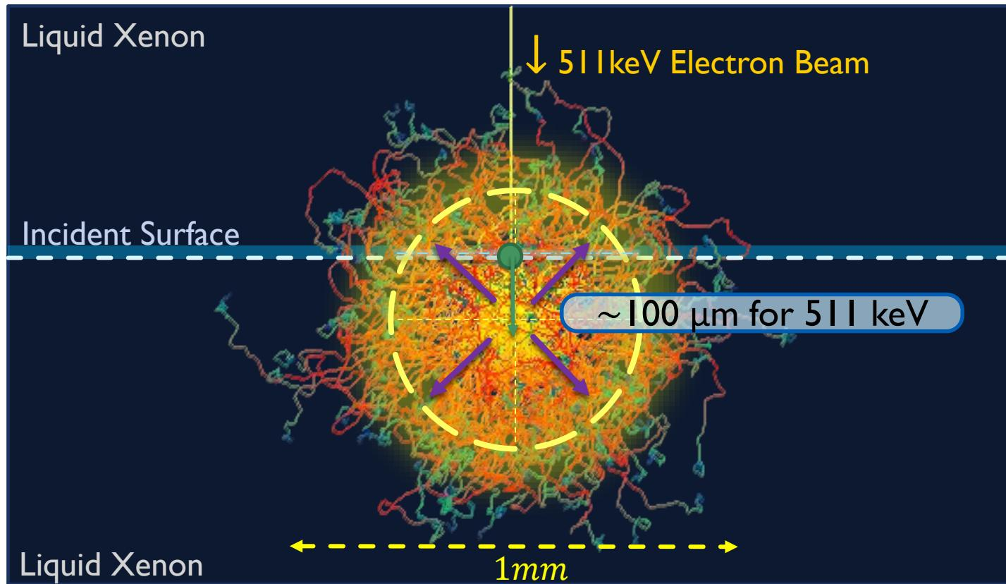
Spread of the electron cloud due to the chaotic trajectory of the primary electrons
