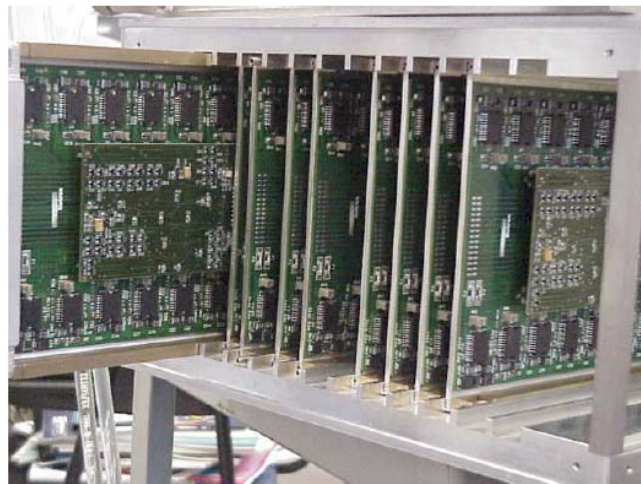
Figure 2: the Regulator Boards, each board is composed by a motherboard and a daughter board
