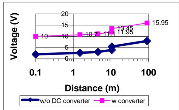
Figure 2: Voltage vs distance from pixel detector on proposed pixel power line.
