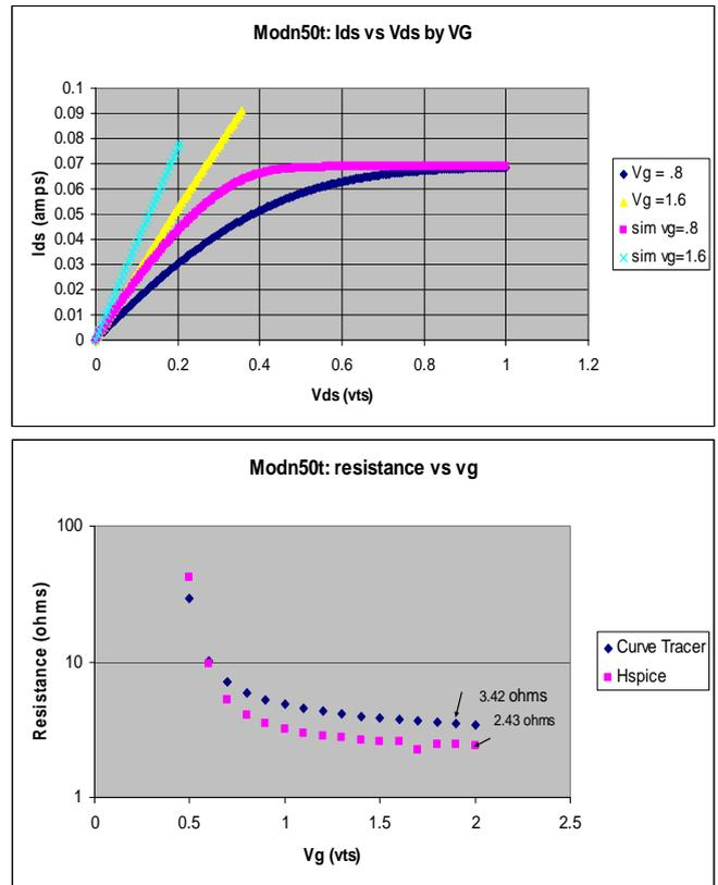
Figure 8: Comparison of (a) the measured and simulated I-V curves for a nmos50t (Modn50t) and (b) the resistance (rds at low vds) vs Vg.
