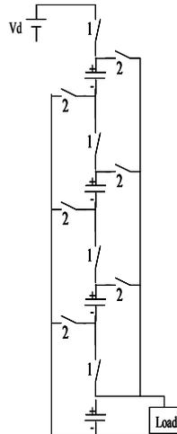
Figure 3: A divide by four switched capacitor circuit.
