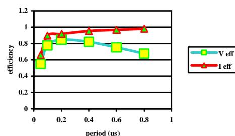
Figure 5: Voltage efficiency and current efficiency vs period.
