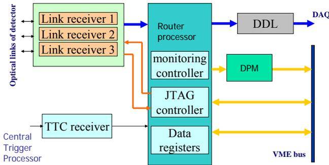
Figure 5: Router architecture
