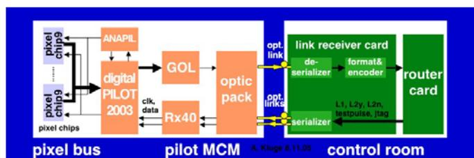
Figure 2: Global readout block diagram
