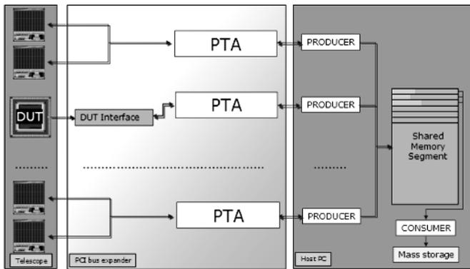
Figure 11: Functional diagram of the test beam DAQ
