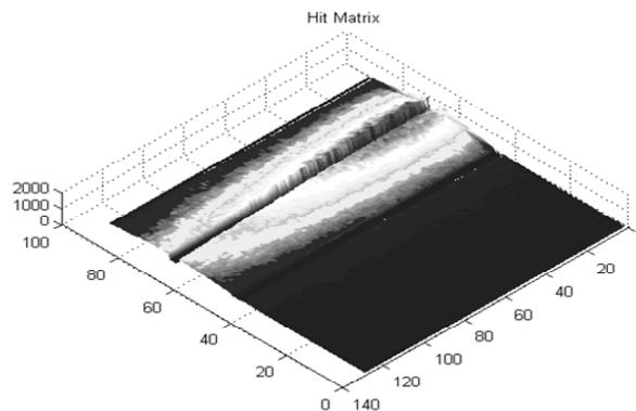
Figure 9: Hit map detail between two FPIX2.1 chips
