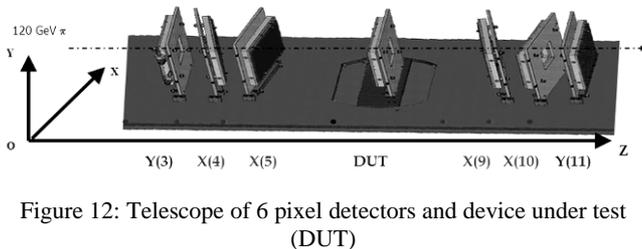
Figure 12: Telescope of 6 pixel detectors and device under test (DUT)
