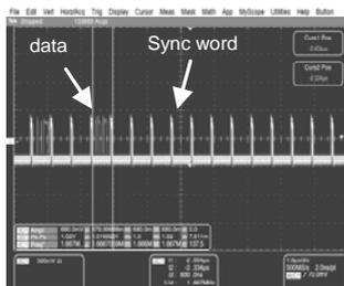
Figure 7: Data output from FPIX2.1 into PTA
