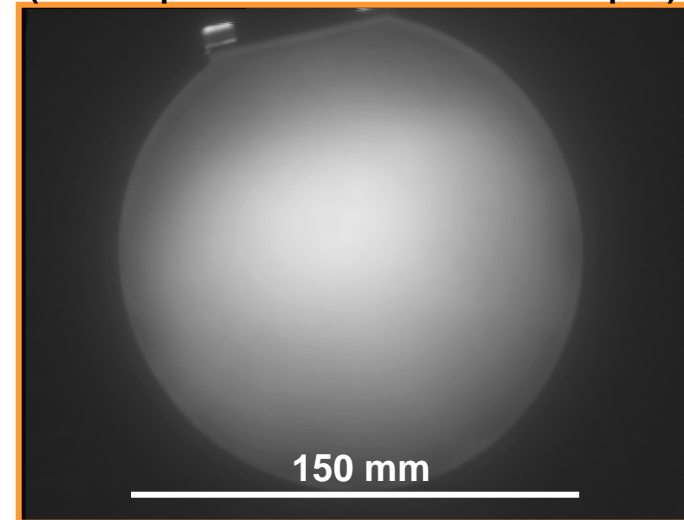
Bonded Wafer-Pair Cross Section
