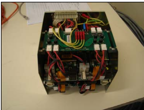
Figure 1: Finger low voltage power supply of the ATLAS Tile Calorimeter.
