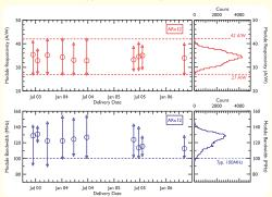
manufacturing facility. This component is the only one to have passed the qualification testing in the first pass, a testament to the high production quality achieved. The two graphs to the left once again show that the production is well centred within the specification window for the gain (upper plot), and in excess of the typical specification on bandwidth (lower plot).
