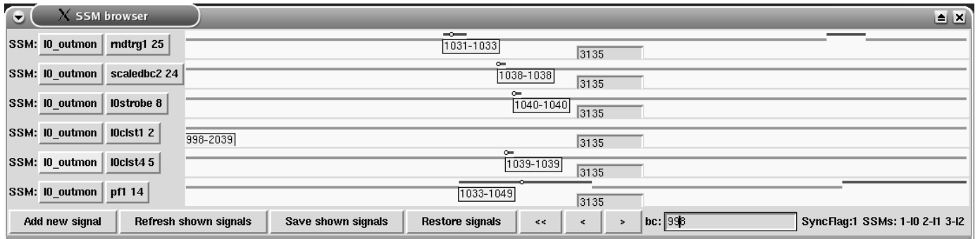
Figure 5: L0 Board snapshot showing the action of past-future protection. The past-future protection circuit is activated by the OR of activity in the signals shown in the first two rows, but only the second row ( scaledbc2 ) is used in the trigger. There are two classes with different output clusters. In one ( l0c1st1 ) there is a past-future protection interval of 15 BC, while in the other ( l0c1st4 ) there is not. The interval when the past-future protection is asserted is shown in the bottom row ( pf1 ), and prevents a trigger from being generated in l0c1st1 .
