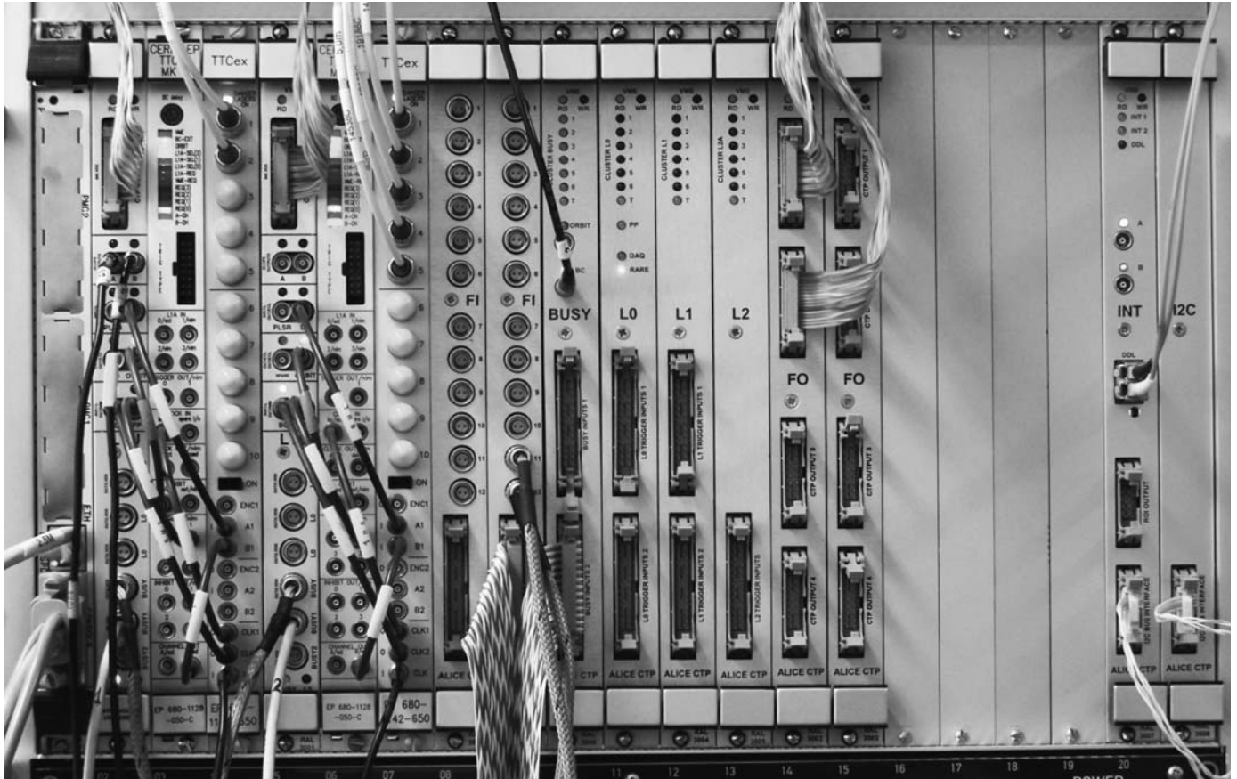
Figure 3: Trigger setup at CERN, showing the full set of CTP boards, together with two sets of TTC interfaces, which transmit to detector emulators about 40m away.
