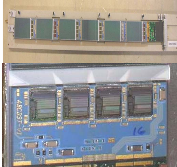
Figure 5: Stave with 6 sensors and the hybrid card.
